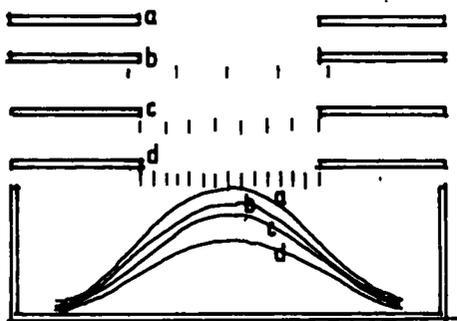
Illumination variation from skylight varying louver spacing as a) no interior louvers. b) spacing = 1h. c) spacing = 2h, Spacing = 4h .
