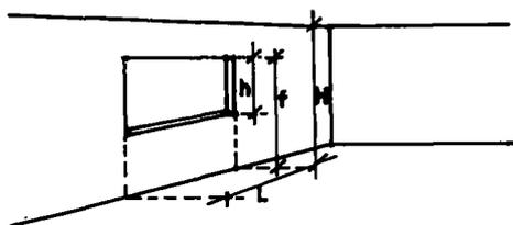
key dimensions for determining  $\bar{H}$ ,  $\bar{V}$ ,  $\bar{M}$  ratios
