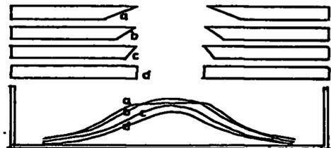
Variation in illumination with horizontal aperture when  $N = 2.1$   $O = 4:1$   $M = \infty:1$  and when well slope is varied as a) 30°, b) 45° c) 60°, d) 90°
