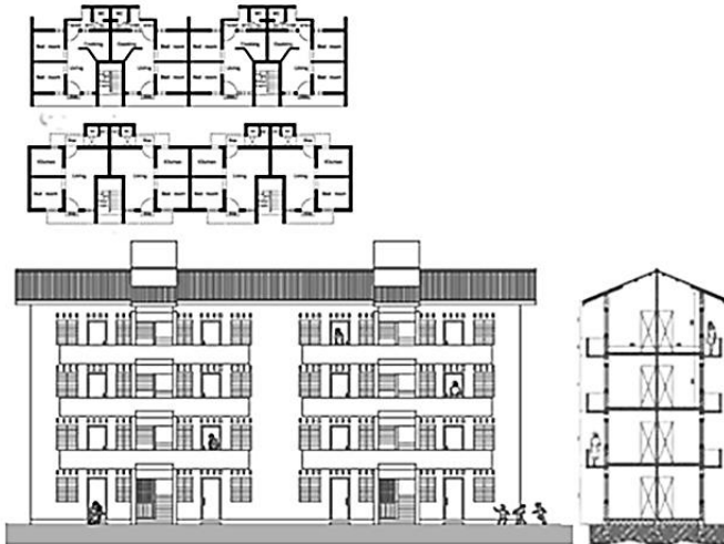
Figure-06: Housing/building types; Typical floor plan; Single bedroom/ 2-unit plan, section, elevation
